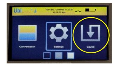
Within the SAVED folder you are able to retrieve any conversations that you have saved to the UbiDuo 3. You also have the capability to copy them to a formatted USB Flash Drive which allows you to transfer the conversation to a computer to be uploaded and stored, printed or archived.
