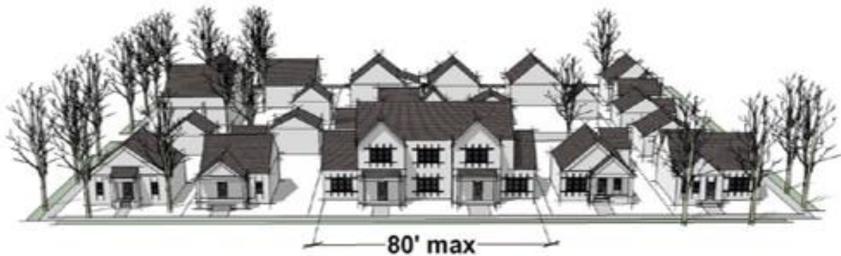
Figure 2-19: Maximum Allowable Length of Multi-Family Residential Structure
