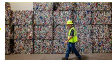
Sorted materials are baled and shipped to customers, where they are used as feedstock for new products.
