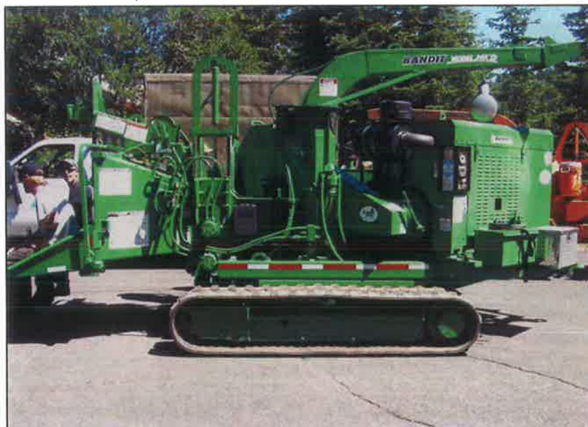
Figure 6.2 – Tracked Chipper. Allows for the chipping of material on-site, reducing the man hours involved with dragging material. This type of equipment still has slope limitations.
