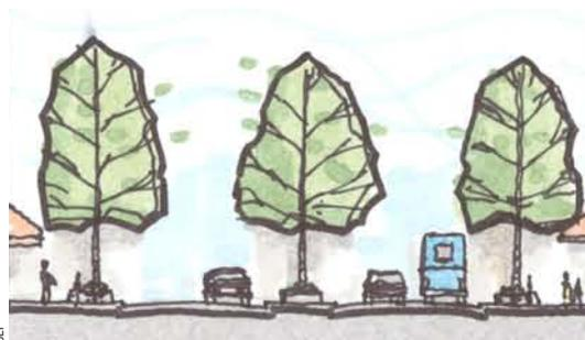
Enhancements depicted in these illustrations depict two lanes of traffic in both directions, in addition to pedestrian developments. Expanding the sidewalks permits addition of medians and trees to increase shading and pedestrian comfort.
