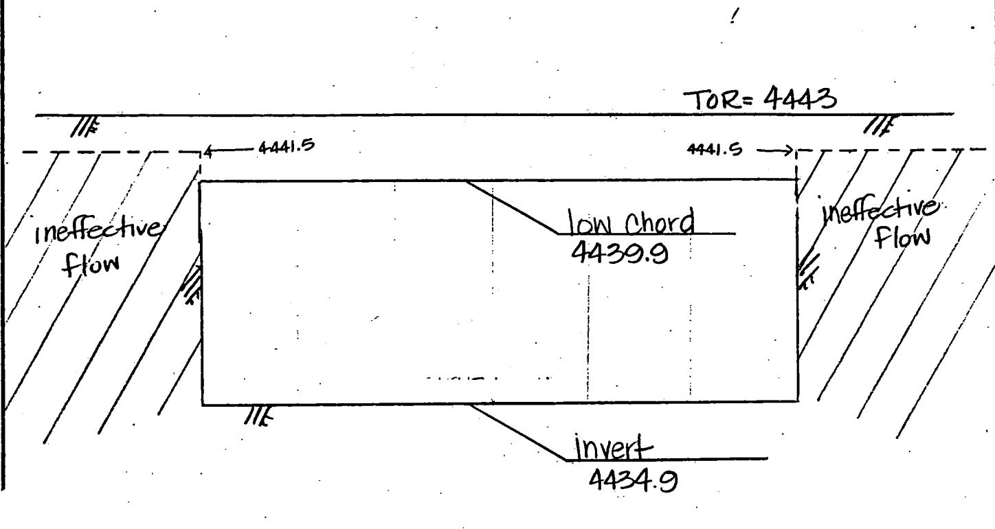
Sketch the upstream face of the structure together with the road profile. Show, at a minimum, the maximum low chord elevation, invert elevation, and minimum top of road elevation.
