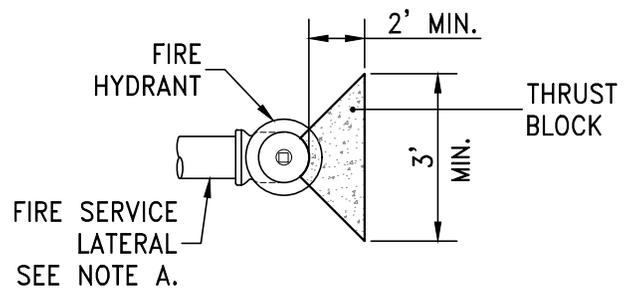
**THRUST BLOCK AT FIRE HYDRANT - PLAN VIEW**
