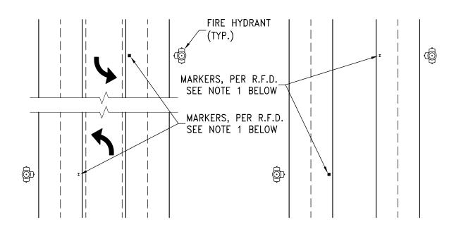
STREETS WITH CENTER TURN LANE, MARKER IS PLACED 8" TO 12" OFF YELLOW SOLID LINE, TO THE SIDE OF THE HYDRANT.
