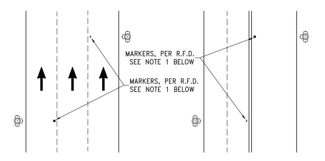
ONE WAY STREETS: MARKER IS PLACED 8" TO 12" OFF LINE IN FIRST LANE, OUT FROM HYDRANT.
