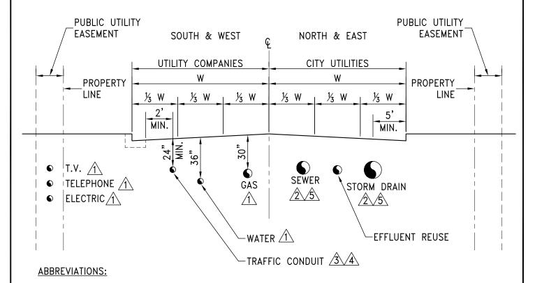
$W = WIDTH FROM CENTERLINE (\mbox{$\P$}) OF ROADWAY TO FRONT FACE OF CURB.$
