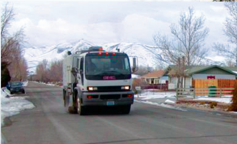
Washoe County street sweeper picks up sand after a snow event, meeting the regional air quality requirement to have all sand picked up within four days of a snow event.
